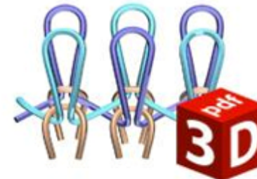
Interlock knitted structure
