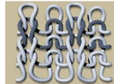
Rib knitted structure
