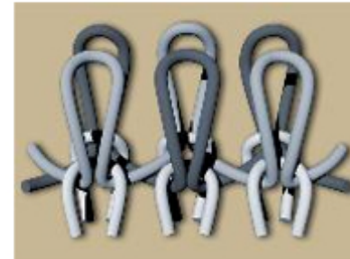
Interlock knitted structure
